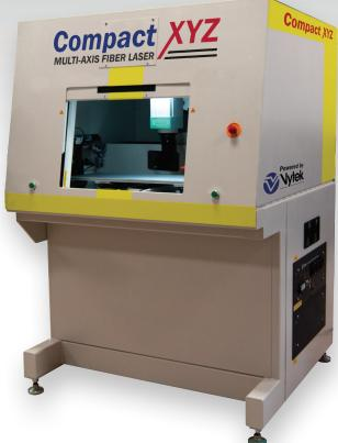
Reliable, turnkey, fiber laser cutting systems designed with flexibility to meet the diverse needs of today's metal fabricator.
