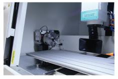
The Compact XYZ series also utilizes a programmable Z axis which makes it ideal for step and repeat applications as well as marking, cutting or welding heights at different levels on a single larger part.
