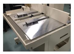
The Compact XYZ base system is a steel structure designed specifically to reduce the effects of the surrounding vibrations while offering a thermally stable support structure. The base is welded and stress relieved then precision ground for high accuracy.
