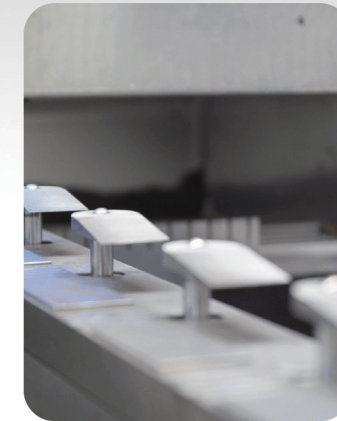
Pneumatic clamps to hold down small substrates
